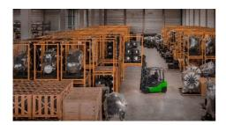
Optimised corner control automatically adjusts drive speed by constantly measuring the steering angle. The higher the steering angle, the more the speed is lowered. Once out of a corner, the speed automatically increases in line with the reduction in steering angle.
