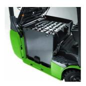
For applications where lead-acid batteries are used, batteries can be swapped in minutes thanks to the optional sideways battery extraction.
