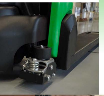
P013i: both the drive wheel and the caster wheels have safe foot protections as standard
